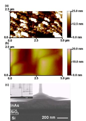
FIG. 2. (Color online) AFM topograph images of InAs on SiO<sub>2</sub>/Si (a) directly after ion-cut induced transfer and (b) after wet etching of damaged layer and OMVPE thin film growth. (c)  $85^{\circ}$  cross-sectional FE-SEM at the base of an InAs NW grown on InAs/SiO2/Si. Inset is FE-SEM image of InAs NWs grown on InAs/SiO<sub>2</sub>/Si.
