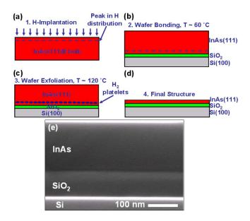
FIG. 1. (Color online) [(a)–(d)] Process flow for ion implantation induced transfer layer to SiO2/Si. (e) Cross-sectional FE-SEM image of the transferred InAs layer to SiO<sub>2</sub>/Si.
