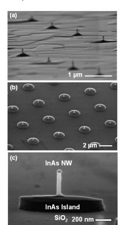
FIG. 3. (a)  $85^{\circ}$  FE-SEM image of ordered InAs NW arrays grown on InAs/SiO<sub>2</sub>/Si. (b)  $45^{\circ}$  angle-view FE-SEM images of vertical and electrically isolated InAs NWs on SiO<sub>2</sub>/Si. (c) Zoom-in FE-SEM image of an InAs NW with an InAs island at its base, sitting on SiO<sub>2</sub> substrate and electrically isolated from other NWs for individual NW addressing.
