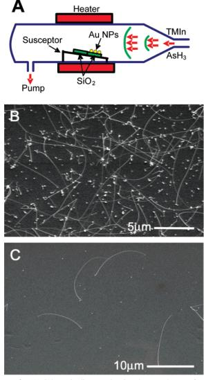
**Figure 2.** (A) Schematic diagram showing the growth setup for the remote effect of the Au nanoparticles in the AsH<sub>3</sub> pyrolysis on SiO<sub>2</sub> substrate. (B) SEM image of NWs grown on the upstream SiO<sub>2</sub> sample with Au nanoparticles on top. (C) SEM image of NWs grown on the downstream SiO<sub>2</sub> sample with no Au nanoparticles on top.
