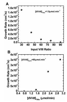
**Figure 5.** (A) NW growth rate as function of the input V/III ratio with constant TMIn flow rate. (B) NW growth rate as function of TMIn flow rate with the  $AsH_3$  flow rate maintained constant.
