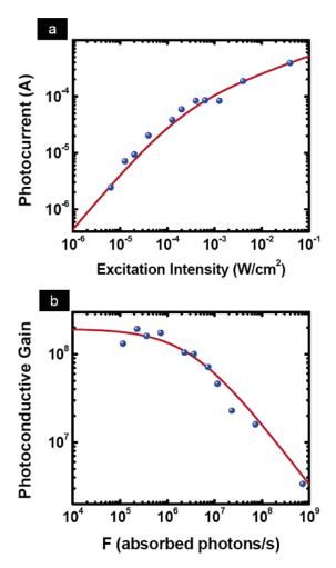
**Figure 3.** (a) Photocurrent of a single ZnO NW device measured as a function of excitation intensity with 5 V applied bias. (b) Estimate of the photoconductive gain relative to the photon absorption rate in the ZnO NW.
