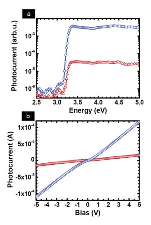
**Figure 5.** (a) Photocurrent spectra of an array of ZnO NWs obtained in air (red triangles) and in vacuum, at  $P \sim 10^{-4}$  Torr (blue circles), with a modulation frequency of 160 Hz and an applied bias of 0.3 V. (b) *I*–*V* characteristics of a single ZnO NW under illumination measured in air (red triangles) and in vacuum, at  $P < 10^{-5}$  Torr (blue circles).
