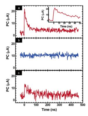
**Figure 6.** Fast transient photocurrent (PC) waveforms of ZnO NWs obtained (a) in air, (b) under vacuum ( $P \sim 10^{-4}$  Torr) and (c) reexposed to air for 1 min after vacuum. The excitation intensity was  $I = 0.3 \ \mu$ J/pulse and the applied bias V = 1 V. Inset of (a) shows the initial photocurrent decay in air, from which a characteristic time of ~20 ns can be inferred.
