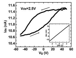
**Figure 6.** Transport properties of a single NW FET based on unintentionally doped GaAs NWs grown on Si (111) substrates. NWs used for devices were grown at 417 °C with  $\chi_{\text{AsH3}} = 1.38 \times 10^{-3}$  and  $\chi_{\text{TMG}} = 5.56 \times 10^{-5}$ . The insert shows a linear  $I_{\text{ds}} - V_{\text{ds}}$  curve at zero gate bias.
