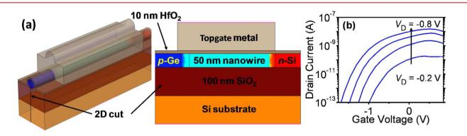
Figure 3. (a) 3D Sentaurus TCAD model and a 2D cut through the midpoint of the wire, with *p*-doped Ge shown as blue and *n*-doped Si as red, dashed line indicates the *p*-Ge/*i*-Si junction; (b) simulated  $I_D - V_G$  characteristics at  $V_D = -0.2$  to -0.8 V in 0.2 V steps, showing good agreement with experimental data.
