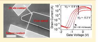
standard nanowire FETs with a good  $I_{ON}/I_{OFF}$  ratio when the source-drain junction is forward-biased. The improved transport in both biasing modes confirms the benefits of utilizing bandgap engineered axial nanowires for enhancing device performance. **KEYWORDS:** SiGe heteronanowire, tunneling field effect transistor, axial heterojunction, VLS growth
