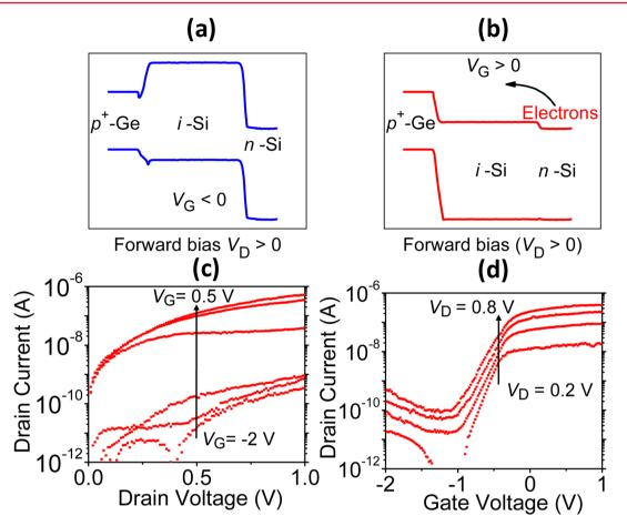
**Figure 4.** (a and b) Energy band diagram of the device in FET working mode where  $V_D > 0$  positive and  $V_G$  modulates thermal injection of carriers: (a) negative  $V_G$  increases the *i*-Si channel barrier, preventing thermal injection of carriers into channel; (b) positive  $V_G$  lowers the *i*-Si barrier, turning on the device; (c) experimental  $I_D - V_D$  at different  $V_G = -2$  to 0.5 V in 0.5 V steps; (d)  $I_D - V_G$  at positive  $V_D = 0.2$  to 0.8 V in 0.2 V steps.
