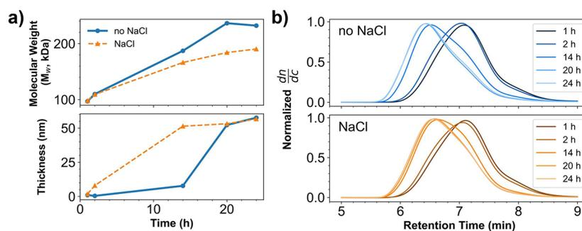
**Figure 2.** Characterization of free PSS and estimation of molecular weight. (a) The molecular weight of the free polymer increases then slows approaching 24 h, likely due to diffusion of oxygen into the system. The thickness of the brushes follows a similar trend. The addition of NaCl (dashed orange) seemed to increase the growth rate of brushes on the surface but did not have significant effect on the dispersity (b) of the free polymer.
