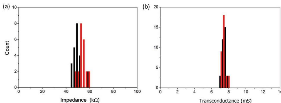
**Figure 2.** a) Histogram showing the distribution in electrode impedance at 1 kHz before (black) and after (red) sterilization. b) Histogram showing the distribution in OECT transconductance before (black) and after (red) sterilization.
