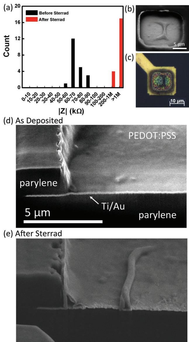
**Figure 3.** a) Impedance histogram at 1 kHz showing mostly open circuit devices after Sterrad sterilization. b) SEM image and c) optical image of a typical PEDOT:PSS microelectrode after Sterrad sterilization, showing clear delamination of the PEDOT:PSS microelectrode from Ti/Au near the edge and near the center after Sterrad sterilization. d,e) FIB cuts of the same electrode before and after sterilization.
