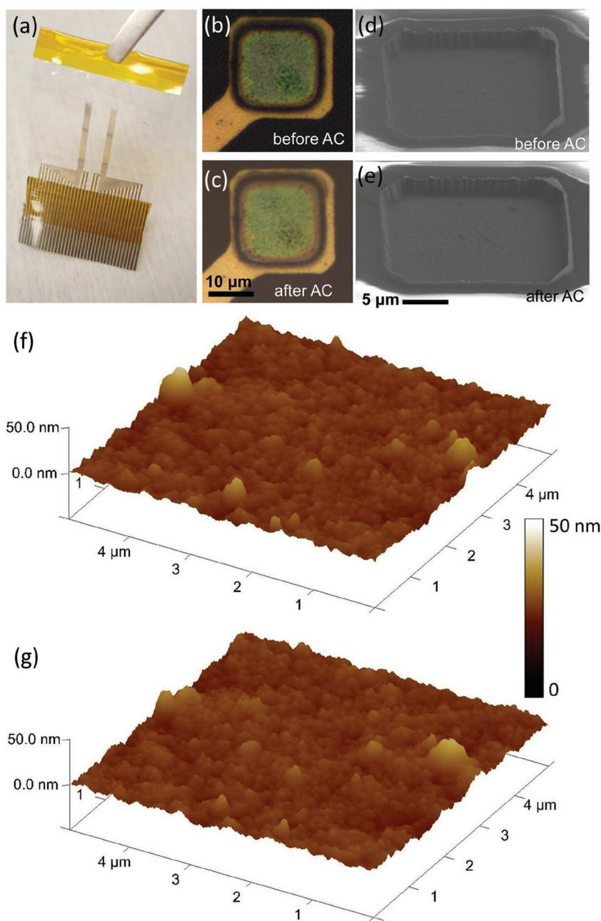
**Figure 1.** a) Picture of test geometry with two arrays, each containing 15 PEDOT:PSS microelectrodes. Optical microscopy images of the same microelectrode b) before and c) after autoclave.  $45^\circ$  angle view SEM images of the same microelectrode d) before and e) after autoclave. AFM topography images on a  $5 \times 5 \mu\text{m}^2$  area at the same location of PEDOT:PSS f) before and g) after autoclave.
