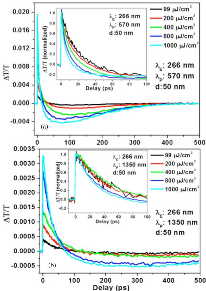
Fig. 4. Pump-fluence-dependent carrier relaxation dynamics in  $d = 50$  nm SiNWs probed at (a) 570 nm and (b) 1350 nm. Insets show the data on a 100 ps timescale with peak amplitudes normalized.
