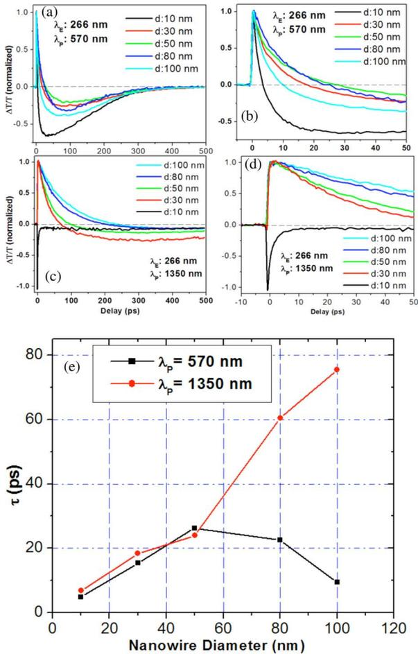
Fig. 2. (a) UV-pump (266 nm), visible-probe (570 nm) measurements on SiNWs of various diameters; (b) data from (a) during the first 50 ps. (c) UV-pump (266 nm), IR probe (1350 nm) measurements on SiNWs of various diameters; (d) data from (c) during the first 50 ps. (e) Graph showing the variation of  $\tau$  with NW diameter at 570 and 1350 nm.
