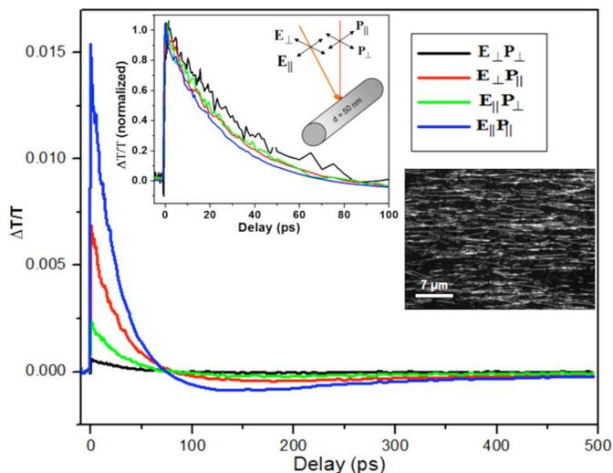
Fig. 3. Polarization-dependent transmission in  $d = 50 \text{ nm}$  SiNWs at a pump fluence of  $400 \mu\text{J}/\text{cm}^2$  and a probe wavelength of 1045 nm. Here, “E” indicates the pump polarization and “P” indicates the probe polarization. The upper left inset shows the corresponding normalized data, and the lower right inset shows an optical microscope image of the NWs after dry transfer onto the sapphire substrate.
