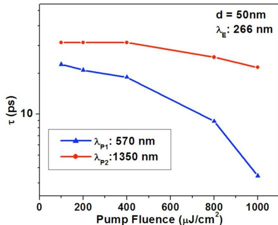
Fig. 5. Plot of  $\tau$  versus pump fluence for  $d = 50$  nm SiNWs probed at 570 and 1350 nm.
