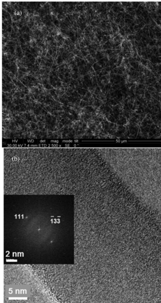
Fig. 1. (a) SEM images of VLS-grown 30-nm SiNWs. (b) TEM image of a 32-nm-diameter SiNW showing (111) lattice fringes. Inset: a fast Fourier transform of the TEM image, indicating the  $\langle 111 \rangle$  growth orientation.
