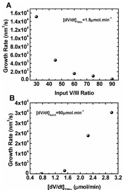
**Figure 5.** (A) NW growth rate as function of the input V/III ratio with constant TMIn flow rate. (B) NW growth rate as function of TMIn flow rate with the AsH<sub>3</sub> flow rate maintained constant.
