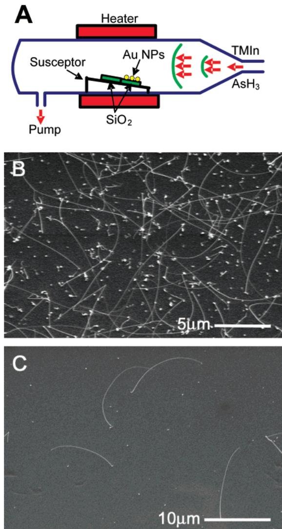
**Figure 2.** (A) Schematic diagram showing the growth setup for the remote effect of the Au nanoparticles in the AsH<sub>3</sub> pyrolysis on SiO<sub>2</sub> substrate. (B) SEM image of NWs grown on the upstream SiO<sub>2</sub> sample with Au nanoparticles on top. (C) SEM image of NWs grown on the downstream SiO<sub>2</sub> sample with no Au nanoparticles on top.
