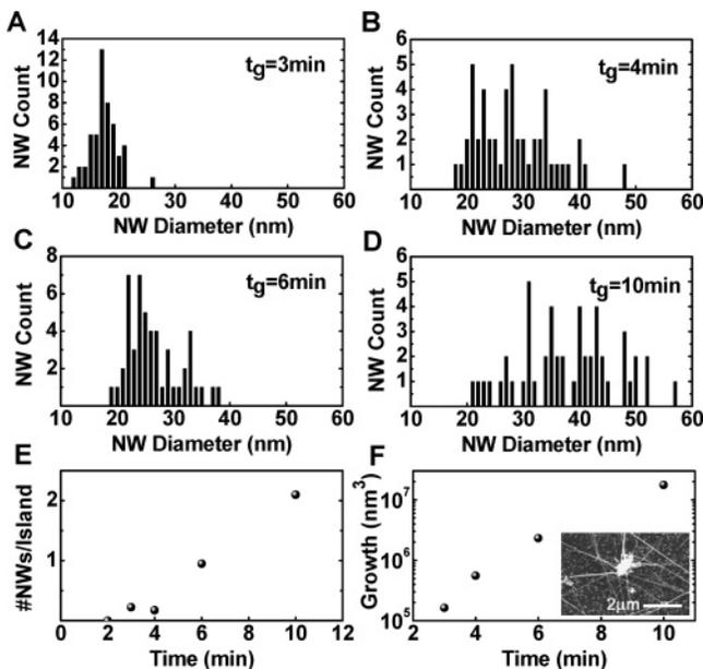
**Figure 3.** (A–D) Histograms of NW diameter variation for different growth times. (E) Number of InAs NWs per single island for different growth times. (F) Total NW growth as function of growth time. Inset is an SEM image of a single InAs island from which several NWs have nucleated.
