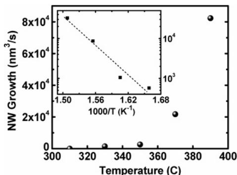
**Figure 4.** NW growth rate as function of growth temperature on the SiO<sub>2</sub> surface. Inset is an Arrhenius plot of the growth rate.
