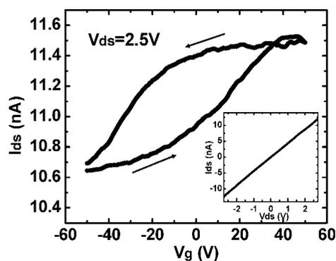
**Figure 6.** Transport properties of a single NW FET based on unintentionally doped GaAs NWs grown on Si (111) substrates. NWs used for devices were grown at 417 °C with  $\chi_{\text{AsH}_3} = 1.38 \times 10^{-3}$  and  $\chi_{\text{TMG}} = 5.56 \times 10^{-5}$ . The inset shows a linear  $I_{\text{ds}}-V_{\text{ds}}$  curve at zero gate bias.
