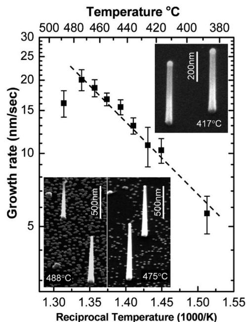
**Figure 3.** Temperature dependence of the growth rate and the morphology of GaAs NWs grown on Si (111) substrates at  $\chi_{\text{AsH}_3} = 1.38 \times 10^{-3}$  and  $\chi_{\text{TMG}} = 5.56 \times 10^{-5}$ . Insets are the tilted 45 °FE-SEM images of GaAs NWs grown for 60 s at 417 °C (upper right), 475 °C (lower right), and 488 °C (lower left).
