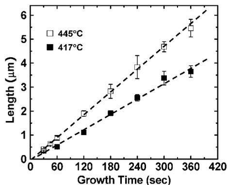
**Figure 2.** Plot of the NW length as a function of time for GaAs NWs grown on Si (111) substrates at 417 °C (solid squares) and 445 °C (hollow squares). The dashed lines are linear fittings to the data. AsH<sub>3</sub> and TMG molar fraction were  $1.38 \times 10^{-3}$  and  $5.56 \times 10^{-5}$ , respectively.
